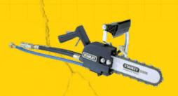
The DS06 is lightweight, powerful and ideal for fast cutting of concrete, reinforced concrete, conduit, brick, stone and other masonry. 13 inch plunge cut capability allows quick cutting of window, door, conduit and duct openings in walls and notching and trimming of concrete pipe. Trigger activated water for lubrication and cooling is ported through the bar and applied at the point where the concrete is being cut.
