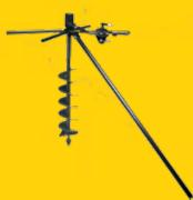
The EA08 features an output torque of 250 ft lb / 339 Nm to handle a wide variety of earth boring applications up to 18 inches / 46 cm in diameter and 42 inches / 107 cm deep. It is configured with 4 handles for two-man operation but can be used by one-man by connecting the torque tube to a power unit or other solid object. An ergonomically designed forward and reverse control valve lever is integrated into the handle. The EA08 accepts 1-3/8 in. hex female augers.
