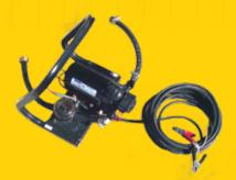
Use the DCP30 Pump to get portable water to your diamond chainsaw. The DCP30 is self priming up to an 8 foot lift and capable of delivering 2.2 gpm at 40 psi and is thermal protected to prevent overheating. A built-in check valve prevents backward flow and maintains pressure after shut-off. The DCP30 is available with battery clips or a marine style DC plug.
